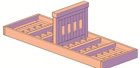
**STEP 4:** Attach diagonal support to bench seat & leg with four deck screws (8" x 2 ½"). *Repeat this step for the other side.*
