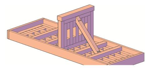
**STEP 5:** Attach bench seat to wall with two bolts (2 ½" x 5/16"), washers & nuts. Tap the bolt all the way into the wood to set it. Then add a washer and nut and lightly tighten. *Repeat this step for the other side*.
