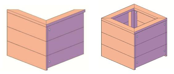
**STEP 2:** Attach bottom to wall with two bolts (3" x 5/16"), washers & nuts. Tap the bolt all the way into the wood to set it. Then add a washer and nut and lightly tighten. *Repeat this step for the other side and for the other planter*.
