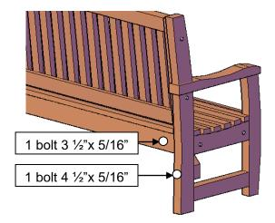
**Step 4:** Attach the front brace to sides, with one bolt (4 ½" x 5/16"), washer & nut per side. Tap the bolt all the way into the wood to set it. Then add a washer and nut and lightly tighten.
