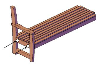
**Step 2:** Attach backrest to sides, with two bolts (3 ½" x 5/16"), washers & nuts per side. Tap the bolt all the way into the wood to set it. Then add a washer and nut and lightly tighten.
