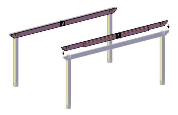
Step 4: Attach the long single supports to the long supports with in-between blocking, use 3/8" X 7 ½" bolts (C).
