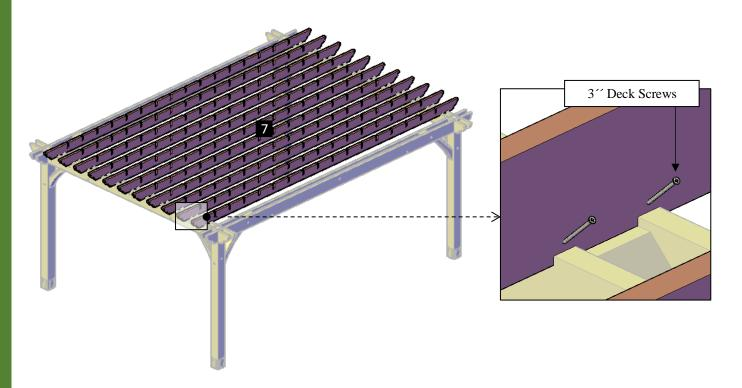
**Step 7:** Attach the short rafters (8) to the long supports and to the long rafters with 3" deck screws (E). Make sure that the rafters fit correctly. Each part has a series of numbers that indicate where to attach the part with the corresponding number
