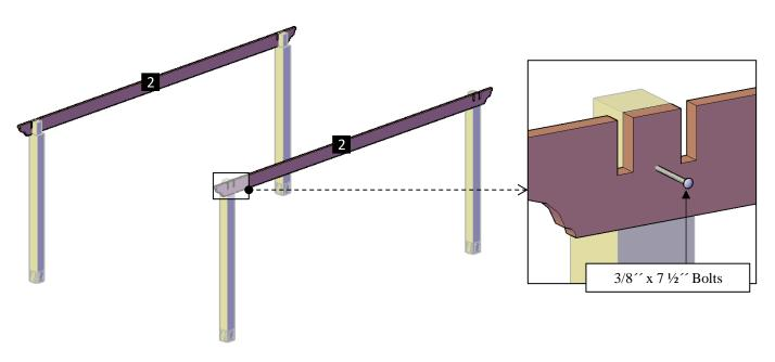
**Step 3:** Put up the long supports with in-between blocking (3), into the post notches as shown and attach to the posts with the single support bolts. Each part has a series of numbers that indicate where to attach the part with the corresponding number.
