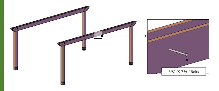
**Step 5:** To attach the short supports (**4,5**) repeat the steps 2 to 4 above. Make sure that the supports fit correctly. Each part has a series of numbers that indicate where to attach the part with the corresponding number.
