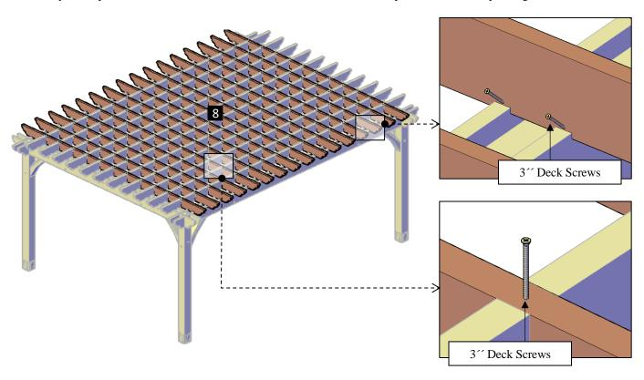
**Step 8:** Finally, use 3" deck screws (**E**) to attach the boots (**9**) to the posts. Each part has a series of numbers that indicate where to attach the part with the corresponding number.
