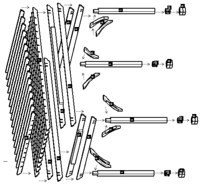
**NOTE:** In order to know where the post needs to be placed, check the numbers on them. If the post is not marked, then place the single Supports on the ground to locate the markings for each post position and clearly set your bearings. ("Don't attach yet, only place them on the ground to begin with").
