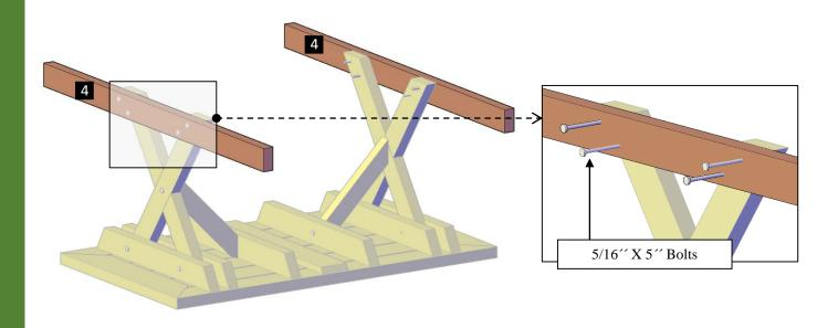
**Step 4:** Attach the bench supports (5) to the table support with 5/16" x 5" bolts (**D**). Each part has a series of numbers that indicate where to attach the part with the corresponding number.
