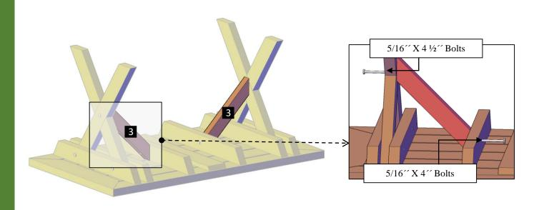
**Step 3:** Use 5/16" x 5" bolts (**D**) to attach one table support (**4**) to the legs. Each part has a series of numbers that indicate where to attach the part with the corresponding number.
