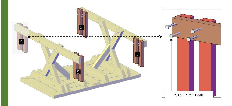
**Step 5:** Place the other table support **(4)** and attach with the bench and table support bolts previously used. Each part has a series of numbers that indicate where to attach the part with the corresponding number.
