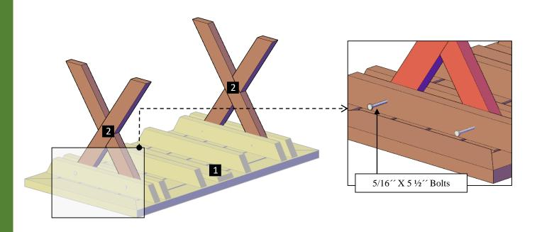
**Step 2:** Attach the knee braces (3) to the tabletop with 5/16" x 4" bolts (B) and to the legs with 5/16" x 4 ½" bolts (C). Each part has a series of numbers that indicate where to attach the part with the corresponding number.
