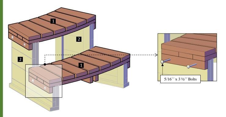
**Step 2:** Attach the central leg (3) to the lower step with  $5/16^{\prime\prime}$  x  $3\frac{1}{2}^{\prime\prime}$  bolts (A). Each part has a series of numbers that indicate where to attach the part with the corresponding number.
