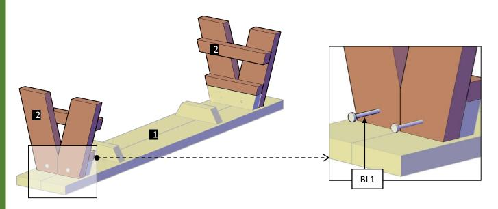
**Step 2:** Attach the diagonal supports (3) to the legs and to the seat with 5/16" x 3 ½" bolts (**BL1**) or 3" deck screws (**DS1**). Each parthas a series of numbers that indicate where to attach the part with the corresponding number.
