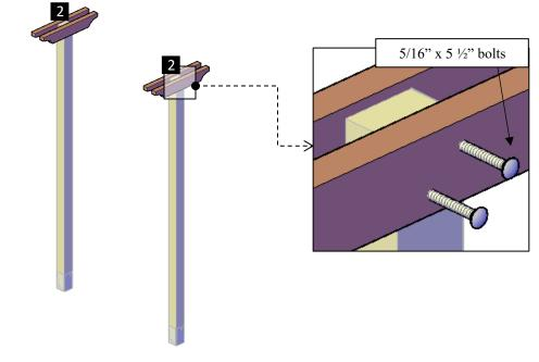
**Step 3:** Attach the main knee braces (5) to the supports with 5/16" x 5  $\frac{1}{2}$ " bolts (C) and to the posts with 3/8" x 7  $\frac{1}{2}$ " bolts (D) with washer and nuts. Each part has a series of numbers that indicate where to attach the part with the corresponding number.
