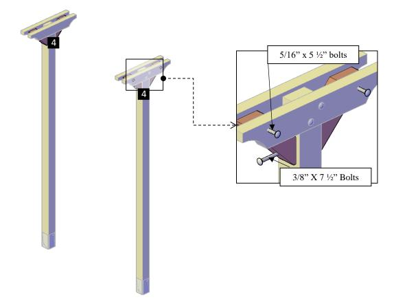
Step 4: Attach the arched rafter (3) to the supports with 5" deck screws (E). Each part has a series of numbers that indicate where to attach the part with the corresponding number.
