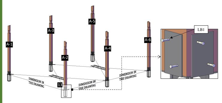
**Step 2:** Attach the single supports **(2)** to the posts with 3/8" x 6 ½" bolts **(BL1)** with washer and nuts. Check the marked numbers on each support and place as drawings shown.
