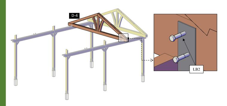
**Step 8:** Attach the secondary knee braces **(8)** to the Roof Trusses with 3/8" x 6 ½" bolts **(BL1)** and to the posts with 3/8" X 9" Bolts **(BL2)** with washer and nuts. Check the marked numbers on each secondary knee brace and place as drawings shown.
