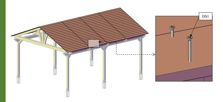
**Step 11:** Attach the roof trims (6) to the roof trusses with 2" deck screws (**DS1**). Check the marked numbers on each roof trims and place as drawings shown.
