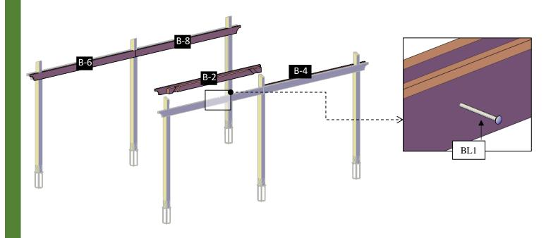
**Step 4:** Attach the main knee braces (7) to the supports with 3/8" x 6 ½" bolts (**BL1**) and to the posts with 3/8" X 9" Bolts (**BL2**) with washer and nuts. Check the marked numbers on each main knee brace and place as drawings shown.
