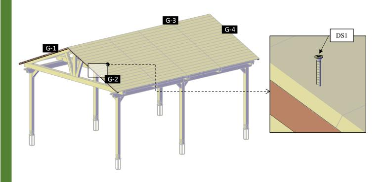
**Step 12:** Attach the fascias (10) to the roof trusses with 2" deck screws (**DS1**). Check the marked numbers on each fascias and place as drawings shown.
