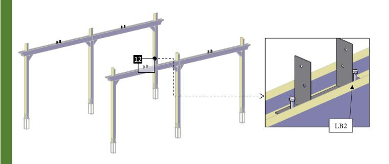
**Step 6:** Attach the perimeter Roof Trusses (4) to the posts with 3/8" x 6 ½" bolts (**BL1**) with washer and nuts to attach the roof trusses (4) to the supports. Check the marked numbers on each roof truss and place as drawings shown.
