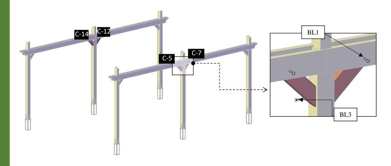
Step 5: Attach the metal plaques (12) to the supports with 3/8" x 3" lag bolts (LB2).
