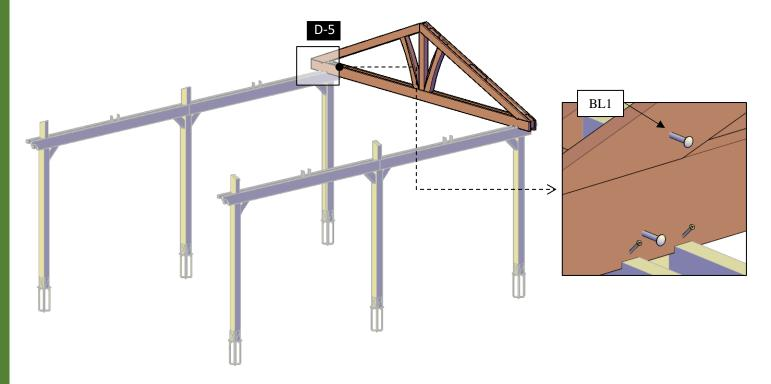
**Step 7:** Attach the roof trusses **(4)** to the metal plaques with 3/8" x 3" lag bolts **(LB2)**. Check the marked numbers on each roof trusses and place as drawings shown.
