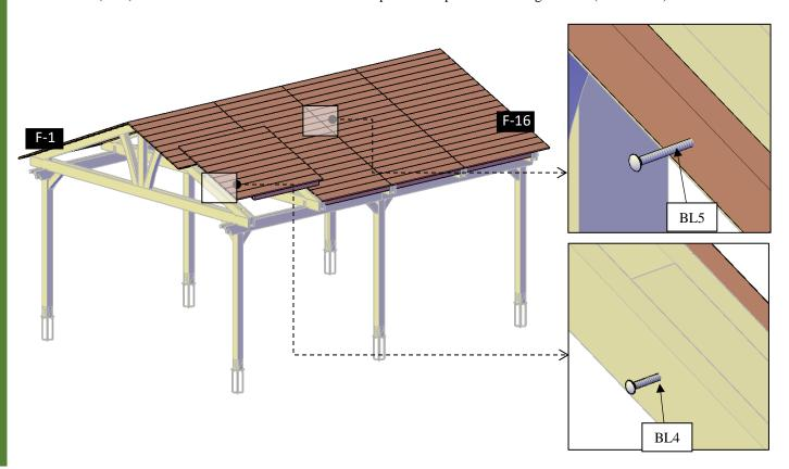
Step 10: Attach the roof boards to the Roof Trusses (4) with 2" deck screws (DS1).
