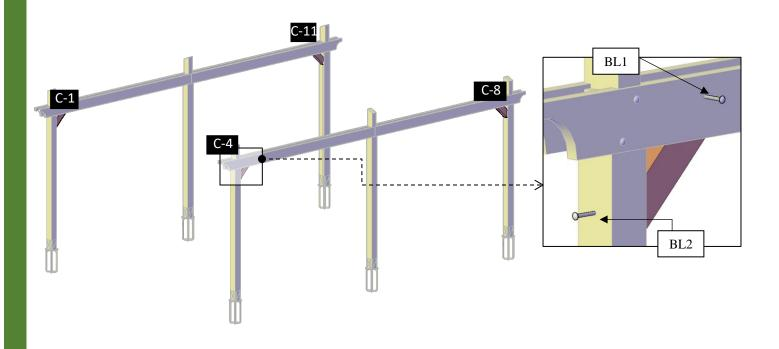
**Step 4:** Attach the central knee braces (7) to the supports with 3/8" x 6 ½" bolts (**BL1**) and to the posts with 3/8" X 12" Bolts (**BL3**) with washer and nuts. Check the marked numbers on each main knee brace and place as drawings shown.
