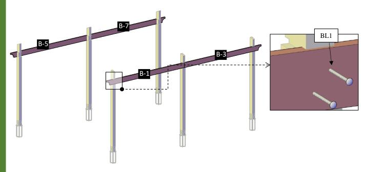
**Step 3:** Attach the single supports to the supports with in-between blocking (3), use 3/8" x 6 ½" bolts (**BL1**) with washer and nuts. After that, return to the bolts described in the step 2 and tighten fully. Check the marked numbers on each support with inbetween blocking and place as drawings shown.
