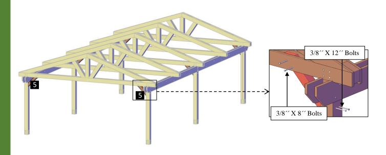
**Step 8:** Attach the main knee braces (6) to the posts with 3/8" x 12" bolts (E) and 3/8" x 16" bolts (F). After that, attach to the supports with 3/8" x 8" bolts (C). Each part has a series of numbers that indicate where to attach the part with the corresponding number.
