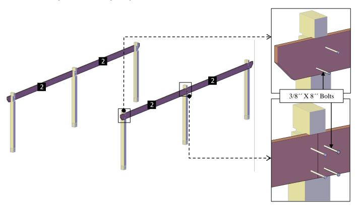
**Step 3:** Put up the supports with in-between blocking (3), into the post notches as shown and attach to the posts with the single support bolts (C). Each part has a series of numbers that indicate where to attach the part with the corresponding number.
