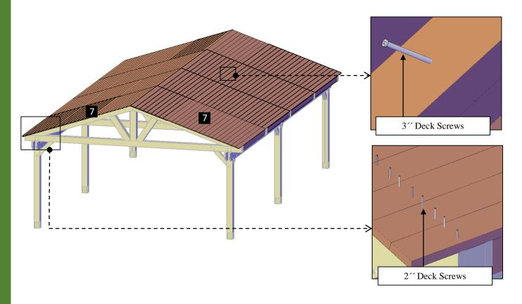
**Step 11:** Attach the roof fascia's **(8)** to the roof panels with 2" deck screws **(I)**. Each part has a series of numbers that indicate where to attach the part with the corresponding number.
