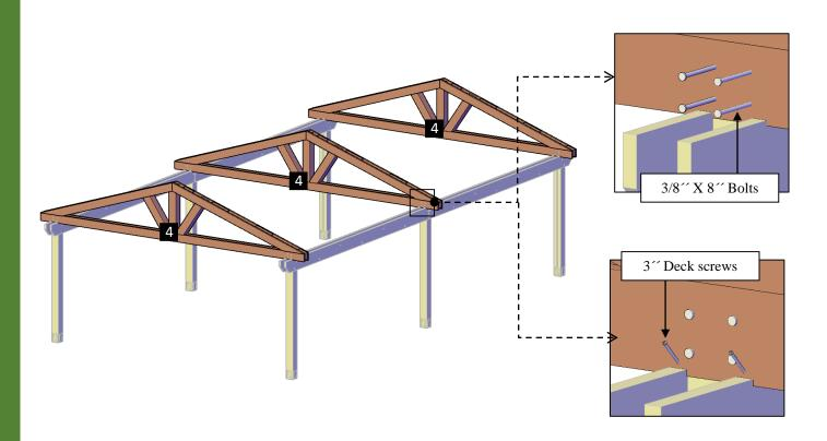
**Step 6:** Attach the central triangles (4) to the supports with 8" x 3" deck screws (**D**). Each part has a series of numbers that indicate where to attach the part with the corresponding number.
