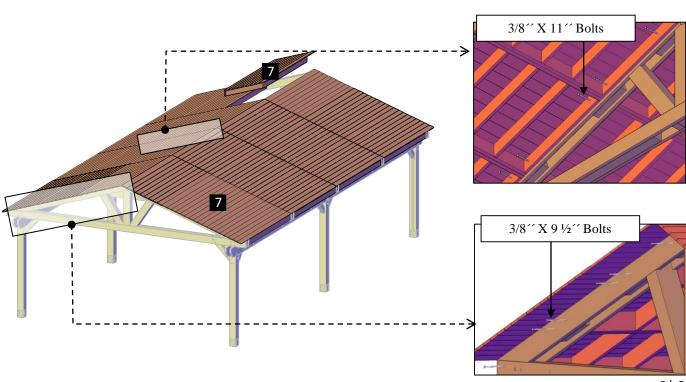
**Step 10:** Attach the roof panels (7) to the triangles with 2" deck screws (**I**). The roof panels will be attached together with 3" deck screws (**D**), as shown below.
