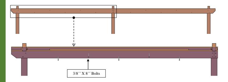
**Step 5:** Attach the triangles (4) to the posts with 3/8" x 8" bolts (C) and to the supports with 8" x 3" deck screws (D). Each part has a series of numbers that indicate where to attach the part with the corresponding number.
