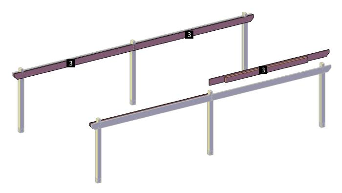
**Step 4:** Attach the single supports to the supports with in-between blocking, use 3/8" x 8" bolts (C). The quantity of bolts depends on the length of the supports.
