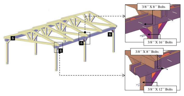
**Step 9:** Use 3/8" x 9 ½" bolts (**G**) to attach the roof panels (**7**) to the perimeter triangles and 3/8" x 11" bolts (**H**) to attach the roof panels (**7**) to the central triangles, as shown below. Each part has a series of numbers that indicate where to attach the part with the corresponding number.
