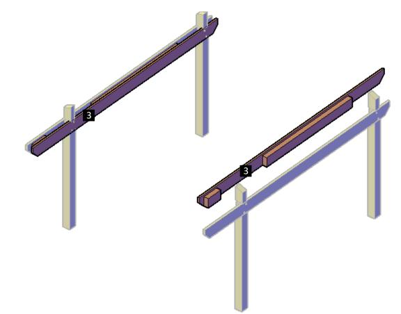
**Step 4:** Attach the single supports to the supports with in-between blocking, use 3/8 x 7  $\frac{1}{2}$  bolts (C). The quantity of bolts depends on the length of the supports.
