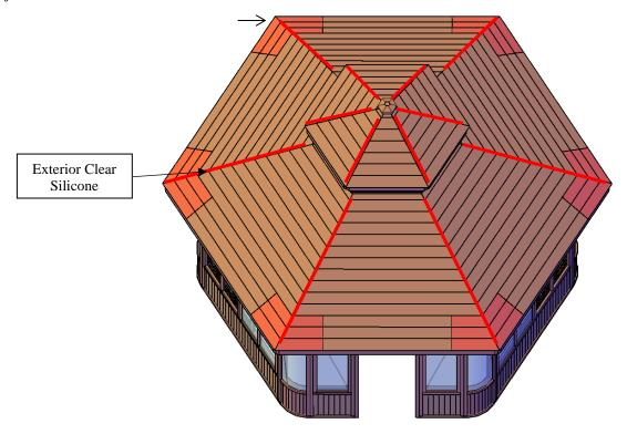
**Step 13:** Measure the roof panels. After that, cut the #30 Felt Roof Deck Protection to those measures. Use staples to attach the #30 Felt Roof Deck Protection to the roof panels.
