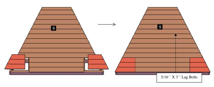
**Step 8:** First Attach four roof panels (9) to the metal plaques with 5/16" x  $4\frac{1}{2}$ " bolts (E). Then, attach the roof panels (9) to the roof frame (10) with 5/16" x  $3\frac{1}{2}$ " bolts (D). Finally, use 3" deck screws (B) to attach the roof panels together. Each part has a series of numbers that indicate where to attach the part with the corresponding number.
