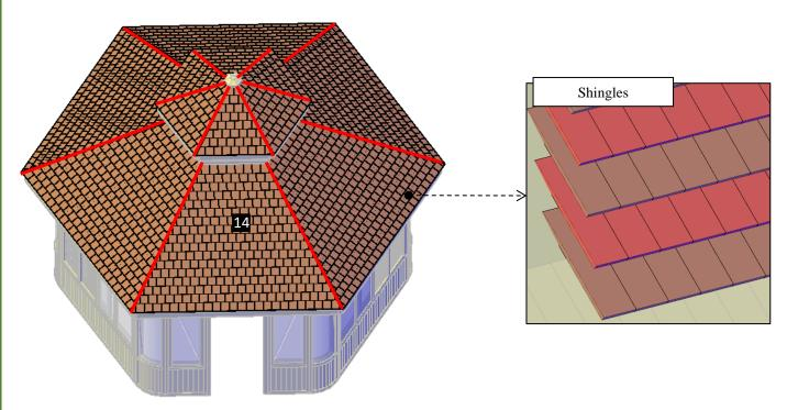
**Step 16:** Finally, use 1 ½ ′′ staples to attach the cap shingles (**15**) and place the doors into the door rail. Each part has a series of numbers that indicate where to attach the part with the corresponding number.
