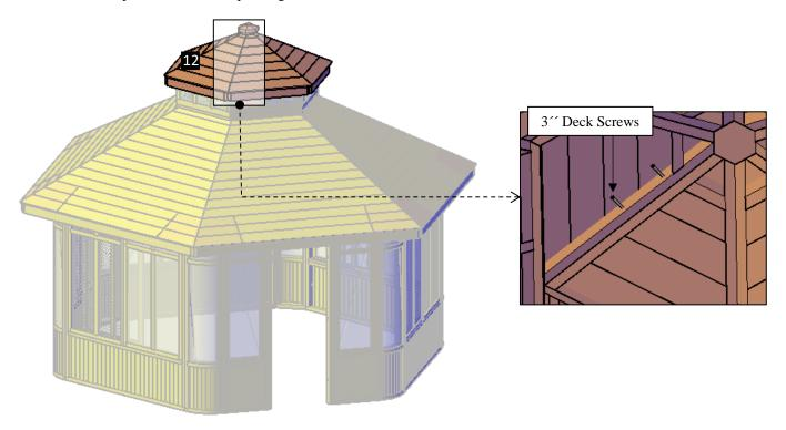
**Step 12:** Place the tables that were removed from the roof panels. After that, put <u>Exterior Clear Silicone</u> on the roof panels joints.
