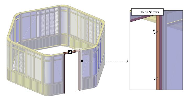
**Step 4:** Attach the supports (8) to the wall panels with 5" deck screws (B). The supports will be attached together with 5/16" x  $5\frac{1}{2}$ " Bolts (C). Each part has a series of numbers that indicate where to attach the part with the corresponding number.
