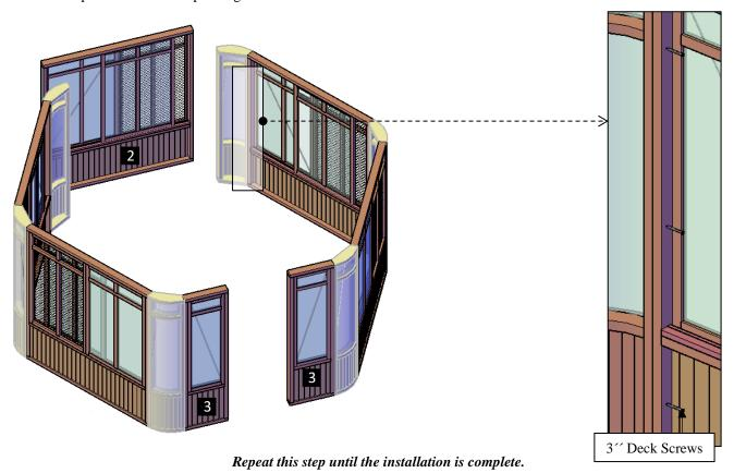
**Step 3:** Attach the door frame (4) to the wall panels with 3" deck screws (A). Each part has a series of numbers that indicate where to attach the part with the corresponding number.
