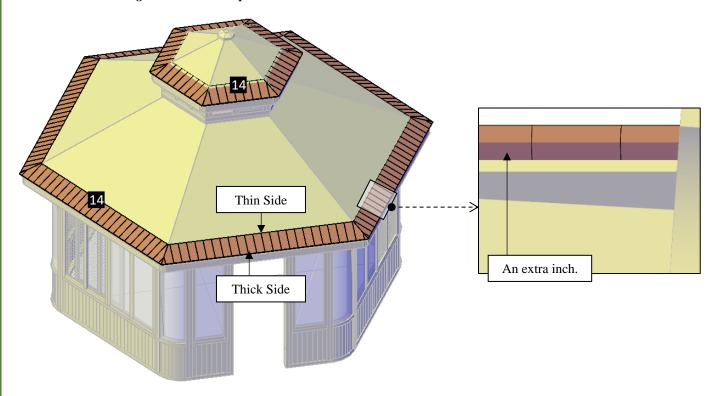
**Step 15:** Put the rest rows of shingles (14) from the bottom to the top and attach with 1 1/4" staples. The overlapping will be at the middle of the shingles. After that, put exterior clear silicone on joints.
