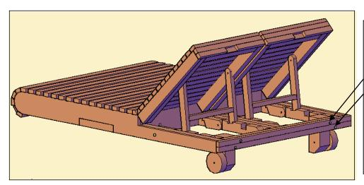
F (Backrest leg) to part A backrest), with two bolts (3/8" x 7"), washers & nuts (into two holes marked "5"). Tap the bolt all the way into the wood to set it. Then add a washer and nut and lightly tighten.
