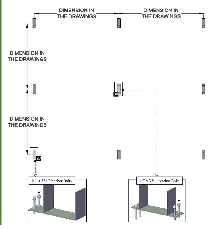
**Step 2:** Set your posts (1), the in-between blockings (3) and the long floor supports (2) in the saddle of the anchor bases. After that, use 5/16 x 3 lag bolts (B) to attach to the anchor bases. Each part has a series of numbers that indicate where to attach the part with the corresponding number.
