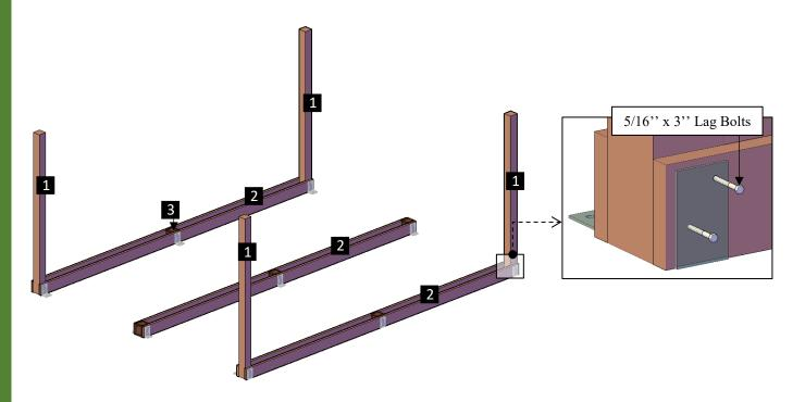
**Step 3:** Attach the short floor supports (4) to the frontal floor supports with 3" deck screws (C). Each part has a series of numbers that indicate where to attach the part with the corresponding number.
