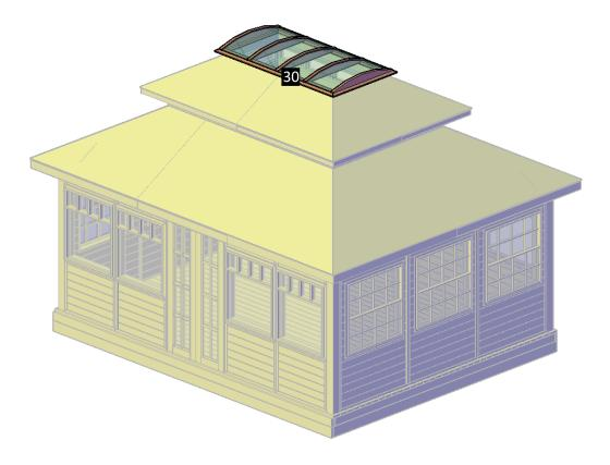
**Step 30:** Use 2'' deck screws (**L**) to attach the roof boards (**31,32**) to the roof panels. Put the boards from the bottom to the top, the overlapping between these boards it will be of ¾''. After that, put <u>exterior clear silicone</u> on the roof boards joints. Each part has a series of numbers that indicate where to attach the part with the corresponding number.
