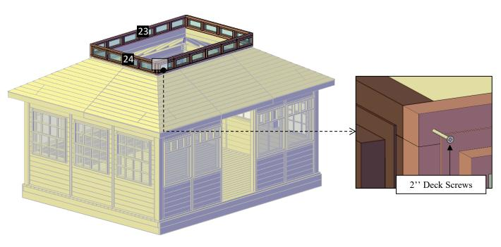
**Step 22:** Use 1 5/8" deck screws (**M**) to attach the roof window trims (**25**) to the roof windows. Each part has a series of numbers that indicate where to attach the part with the corresponding number.
