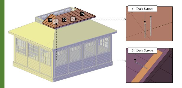
**Step 25:** Use 6'' deck screws (N) to attach the second roof frame (26,27) to the second roof panels. Each part has a series of numbers that indicate where to attach the part with the corresponding number.
