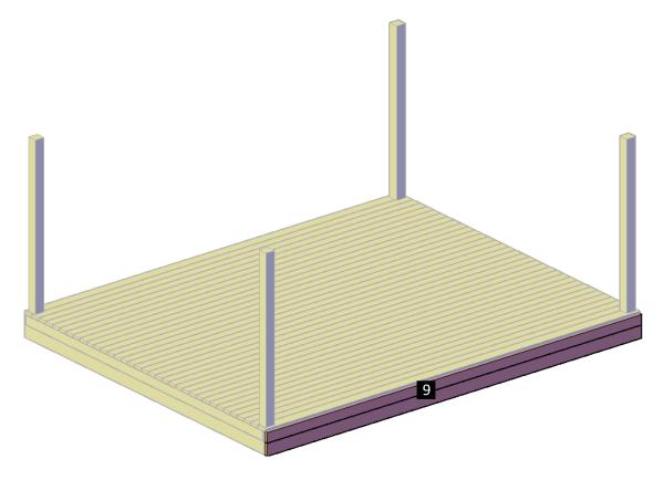
**Step 8:** Attach the back wall panels (10) to the post with 3/8" x 4" lag bolts (**E**). Then, attach the wall panels together with 3/8" x 3" lag bolts (**F**). Each part has a series of numbers that indicate where to attach the part with the corresponding number.
