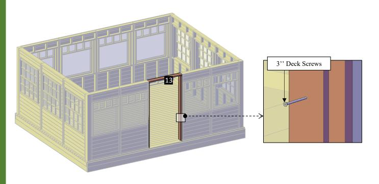
**Step 12:** Attach the wall panels to the roof supports (**14,15**) with 3/8" x 3" lag bolts (**F**). After that, use 3/8" x 8" lag bolts (**G**) to attach the roof supports together. Each part has a series of numbers that indicate where to attach the part with the corresponding number.
