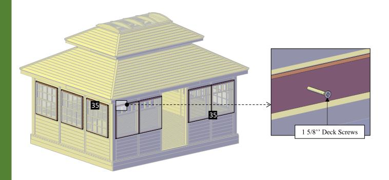
**Step 33:** Finally, with the deck screws included attach the doors (36) to the door frame. Each part has a series of numbers that indicate where to attach the part with the corresponding number.
