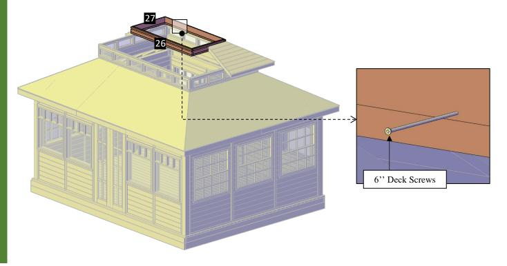
**Step 26:** To attach the rest of second roof panels, repeat the steps 24 and 25. Each part has a series of numbers that indicate where to attach the part with the corresponding number.
