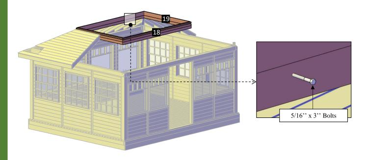
**Step 19:** To attach the rest of roof panels, repeat the steps 17 and 18. Each part has a series of numbers that indicate where to attach the part with the corresponding number.
