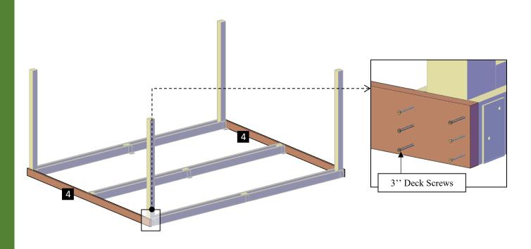
**Step 4:** Use 3" deck screws (C) to assemble the floor frame (5,6). Each part has a series of numbers that indicate where to attach the part with the corresponding number.
