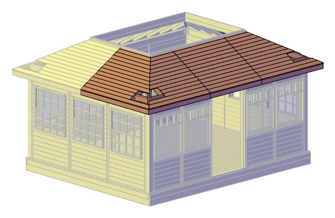
**Step 20:** Place the tables that were removed from the corner roof panels. After that, put the exterior clear silicone on the perimeter of the roof frame and on the roof panels join.
