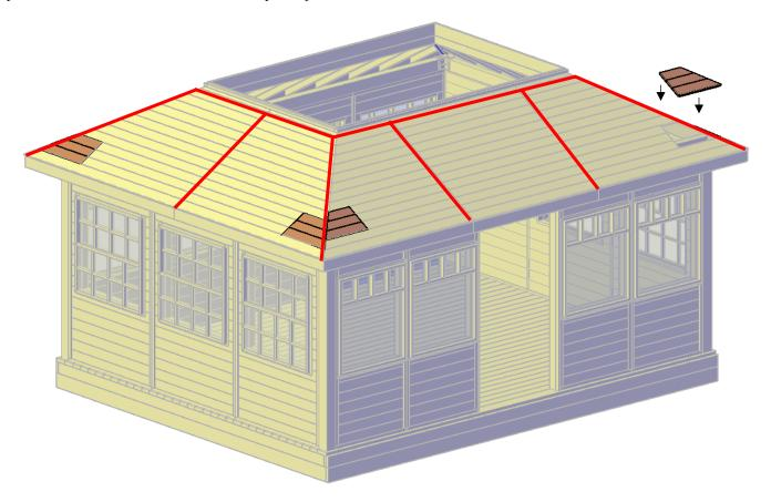
**Step 21:** Use 2" deck screws (**L**) to attach the roof windows (**23,24**) to the roof frame. The roof windows will be attached together with 2" deck screws. Each part has a series of numbers that indicate where to attach the part with the corresponding number.
