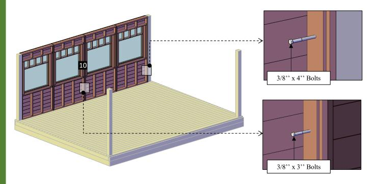
**Step 9:** Attach the lateral wall panels (11) to the post with 3/8" x 4" lag bolts (E). Then, attach the wall panels together with 3/8" x 3" lag bolts (F). Each part has a series of numbers that indicate where to attach the part with the corresponding number.
