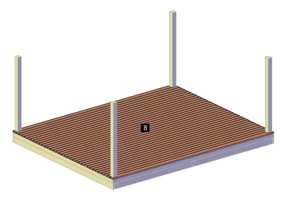
**Step 7:** Attach the floor fascia boards (9) to the floor frame with 2 ½" deck screws (**D**). Each part has a series of numbers that indicate where to attach the part with the corresponding number.
