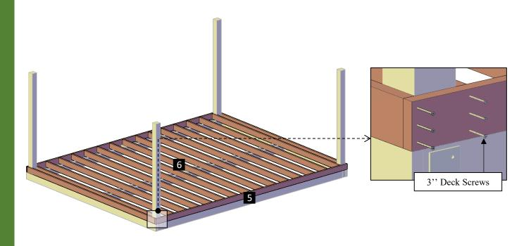
**Step 5:** Attach the floor frame spacers (7) to the floor frame with 3" deck screws (C). Each part has a series of numbers that indicate where to attach the part with the corresponding number.
