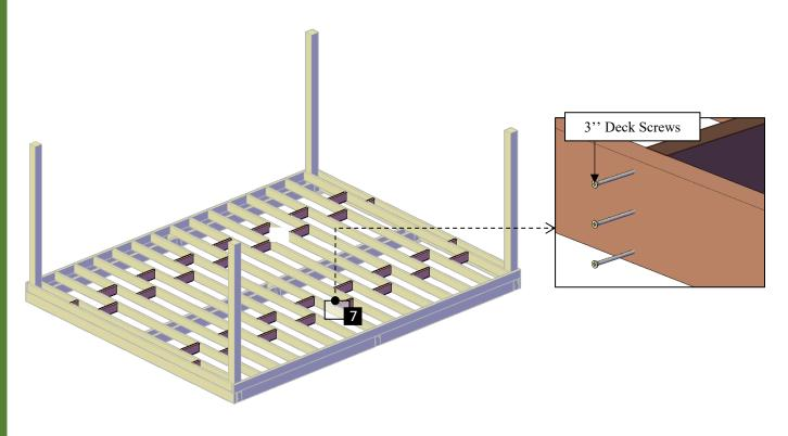
**Step 6:** Use 3" deck screws (**C**) to attach the floor boards (**8**) to the floor frame. Each part has a series of numbers that indicate where to attach the part with the corresponding number.
