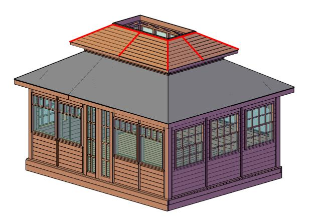
**Step 28:** First, measure the second roof panels. After that, cut the #30 Felt Roof Deck Protection to those measures. Use staples to attach the #30 Felt Roof Deck Protection to the second roof panels.
