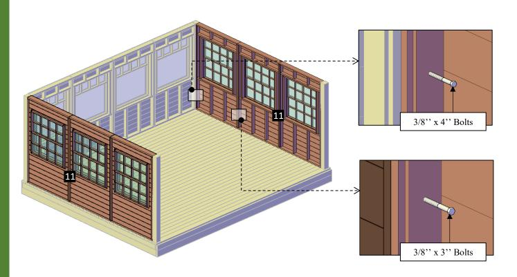
**Step 10:** Attach the frontal wall panels (12) to the post with 3/8" x 4" lag bolts (**E**). Then, attach the wall panels together with 3/8" x 3" lag bolts (**F**). Each part has a series of numbers that indicate where to attach the part with the corresponding number.
