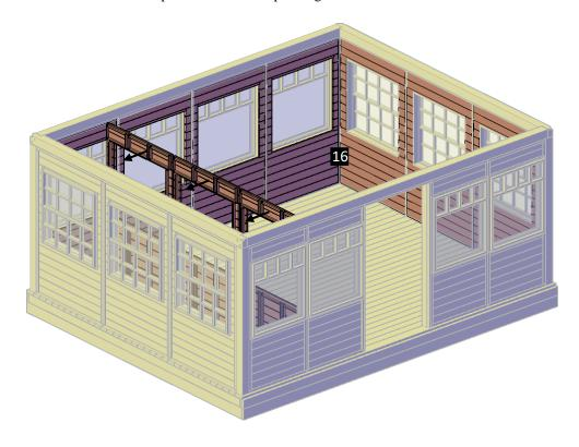
**Step 14:** Attach the Angles (39) and the diagonal bases (40) to the roof supports with 5/16" x 3" lag bolts (B). Each part has a series of numbers that indicate where to attach the part with the corresponding number.
