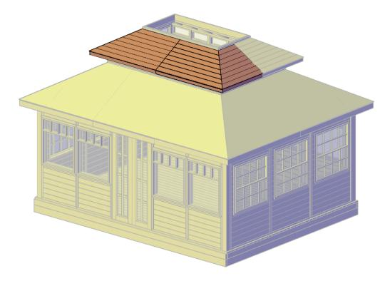
Step 27: Put the exterior clear silicone on the perimeter of the second roof frame and on the second roof panels join.
