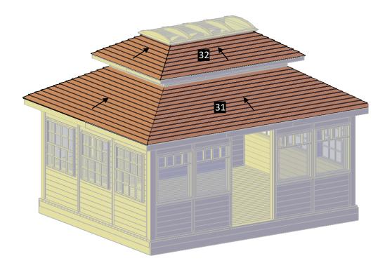
**Step 31:** Use  $3^{\prime\prime}$  deck screws (C) to attach the roof trims (33,34) to the skylight and to the second roof frame. After that, use  $3/8^{\prime\prime}$  x  $4^{\prime\prime}$  lag bolts (J) to attach to roof boards. Each part has a series of numbers that indicate where to attach the part with the corresponding number.
