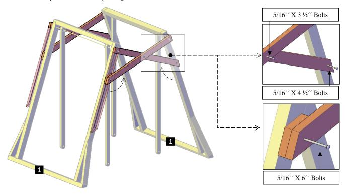
**Step 2:** Assemble the base leg support (2) to the legs supports with  $5/16^{\prime\prime}$  x  $3^{\prime\prime}$  bolts (**D**) as shown. Each part has a series of numbers that indicate where to attach the part with the corresponding number.
