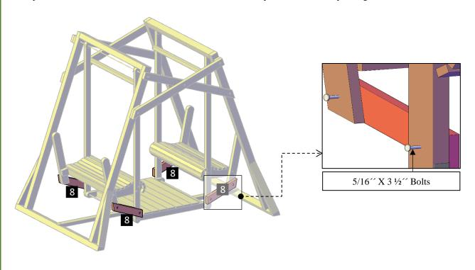
**Step 9:** Attach the bench backrests (9) to the bench seats with  $5/16^{\prime\prime}$  x  $3\frac{1}{2}^{\prime\prime}$  bolts (C). Each part has a series of numbers that indicate where to attach the part with the corresponding number.
