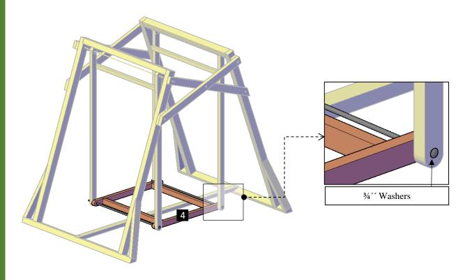
**Step 5:** Later the **Step 4** put the removable floor (5) over the floor frame. Each part has a series of numbers that indicate where to attach the part with the corresponding number.
