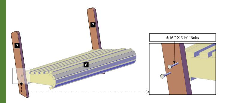
**Step 7:** Use 5/16" x 3 ½" bolts (**C**) to attach the bench seat (**6**) to the straps in the legs supports. Each part has a series of numbers that indicate where to attach the part with the corresponding number.
