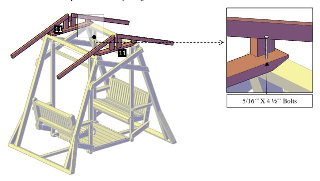
**Step 12:** Attach the roof panels (12) to the triangles with  $5/16^{\prime\prime}$  x  $4^{\prime\prime}$  bolts (E). Each part has a series of numbers that indicate where to attach the part with the corresponding number.
