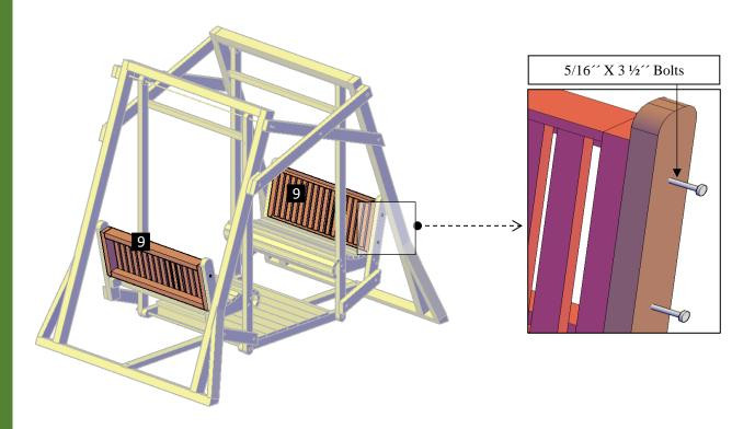
**Step 10:** Use 5/16" x 3 ½" bolts (**C**) to attach the bench arms (**10**) to the straps in the legs supports and to the bench seats. Each part has a series of numbers that indicate where to attach the part with the corresponding number.
