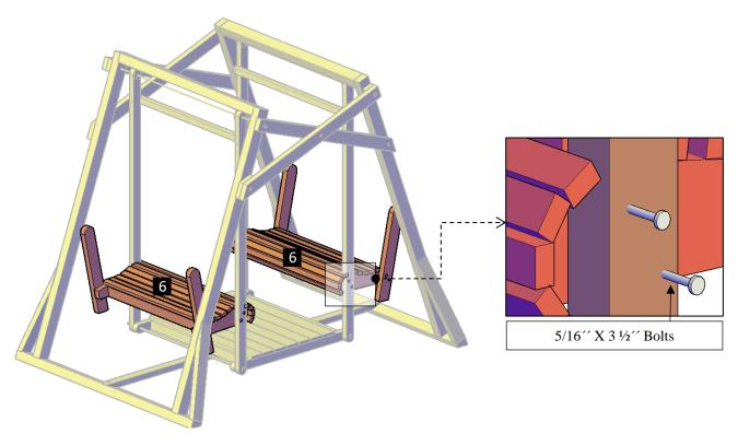
**Step 8:** Attach the short bench supports (8) to the bench seats and to the straps in the legs supports with 5/16" x 3 ½" bolts (C). Each part has a series of numbers that indicate where to attach the part with the corresponding number.
