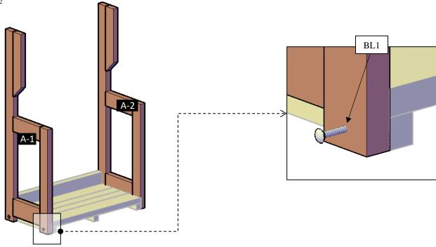
**Step 2:** Attach the Parquet shelve (2) to the legs (1), use 3/8" x 4 ½" bolts (**BL1**) with washer and nuts. Check the marked numbers on each parquet shelve and place as drawings shown.
