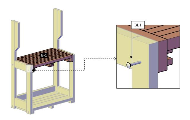
**Step 3:** Attach the shelves (5) to the legs (1) with 3/8" x 4  $\frac{1}{2}$ " bolts (**BL1**) with washer and nuts. Check the marked numbers on each shelve and place as drawings shown.
