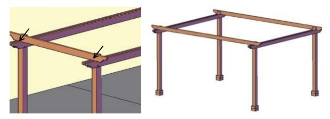
**Step 4.** Attach secondary knee brace to post & rafter with two bolts, washers & nuts. (Match numbers). Tap the bolt all the way into the wood to set it, then add a washer and nut and lightly tighten. Repeat this step with the other end arch.
