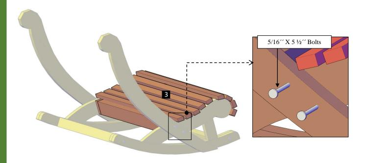
**Step 3:** Use 5/16 'x  $3\frac{1}{2}$ ' bolts (**A**) to attach the armrests (**4**) to the legs and 5/16 'x  $5\frac{1}{2}$ ' bolts (**B**) to attach to the seat. Each part has a series of numbers that indicate where to attach the part with the corresponding number.
