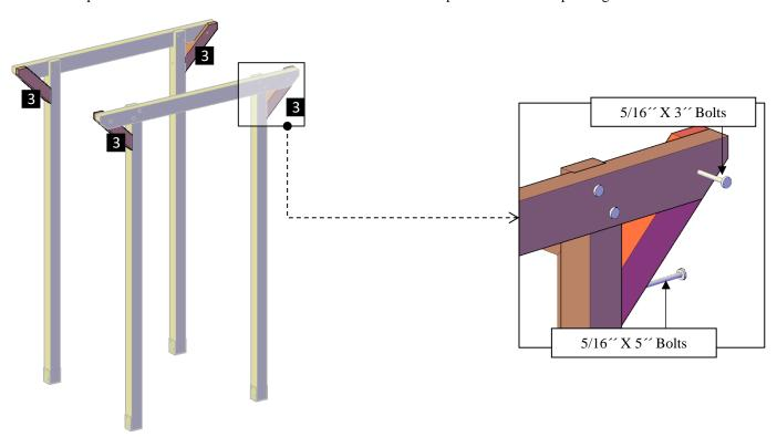
**Step 4:** Attach the trellis wall panels (4) to the posts with 5/16" x  $4\frac{1}{2}$ " bolts (**E**) washers & nuts. Each part has a series of numbers that indicate where to attach the part with the corresponding number.
