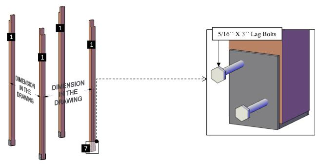
**Step 2:** Attach the supports (2) to the posts with 5/16" x 3" bolts (C) washers & nuts. Tap the bolt all the way into the wood to set it. Then add a washer and nut and lightly tighten. Each part has a series of numbers that indicate where to attach the part with the corresponding number.
