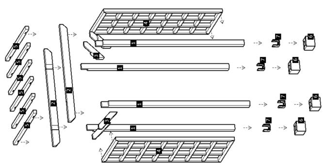
**NOTE:** In order to know where the posts need to be placed, check the numbers on them. If the post is not marked, then place the arched roof timbers on the ground to locate the markings for each post position and clearly set your bearings. ("Don't attach yet, only place them on the ground to begin with").
