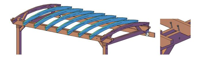
**Step 9.** Attach the center slat atop the arches with deck screws. The slats have notches to fit into the rafters.
