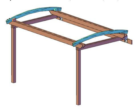
**Step 7.** Attach the 22" diagonal braces to dual supports and posts. Attach the 29" diagonal braces to end rafters and posts with bolts, washer and nuts as shown below:
