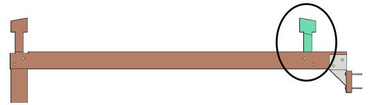
**Step 5.** Attach the main dual supports to the posts and mini posts with 2 bolts (6" x 3/8") washers & nuts per connection. This beam must be in the interior of the support and bolted after you attach the supports to posts as shown below:
