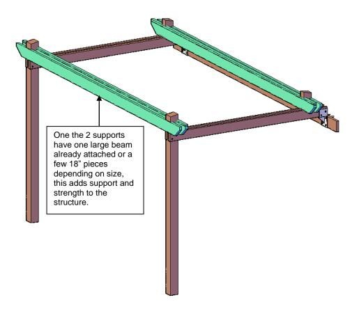
**Step 6.** Attach the end rafters to the posts with one bolt (6" x 3/8") washers & nuts per connection.
