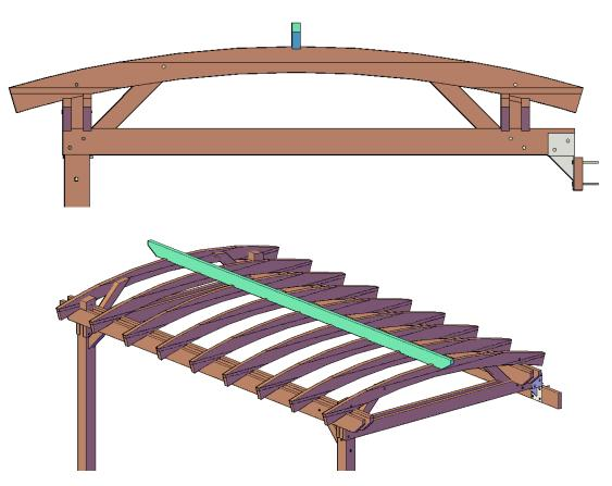
**Step 10.** Attach the lattice panels and the rest of the slats on both sides of this first slat.
