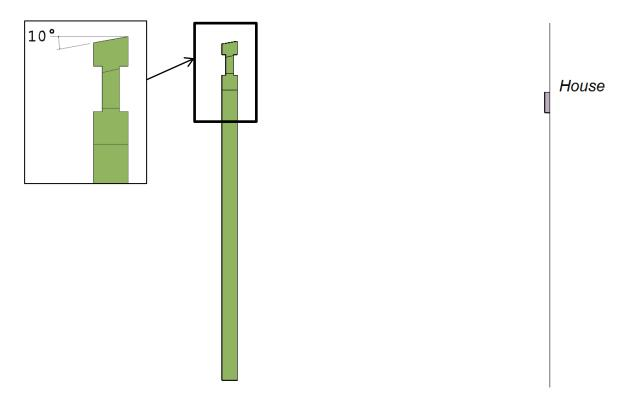
**Step 2.** Attach the ledger board to the wall. The distance from the ground to the bottom of the ledger must be 7'-10 3/4" (see approved drawings-Revision G). Using 3/8" lag screws @ 16" o.c. with 3" min. penetration into the wall studs.
