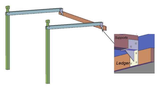
**Step 4.** Attach the mini posts to these supports with 2 bolts (6" x 3/8") washers & nuts.
