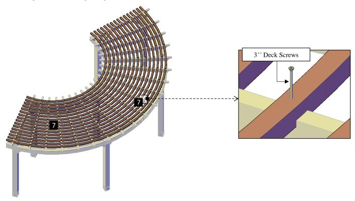
**Step 11:** Finally, attach the boots (8) to the posts with 3" deck screws (I). Each part has a series of numbers that indicate where to attach the part with the corresponding number.
