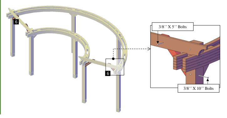
**Step 9:** Attach the rafters **(4)** to the supports with 3" deck screws **(I)**. Each part has a series of numbers that indicate where to attach the part with the corresponding number.
