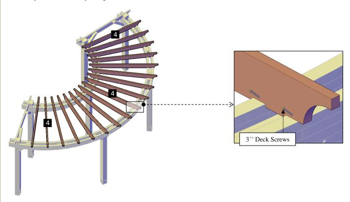
**Step 10:** Use 3" deck screws (**I**) to attach the Slats (**7**) to the rafters. Each part has a series of numbers that indicate where to attach the part with the corresponding number.
