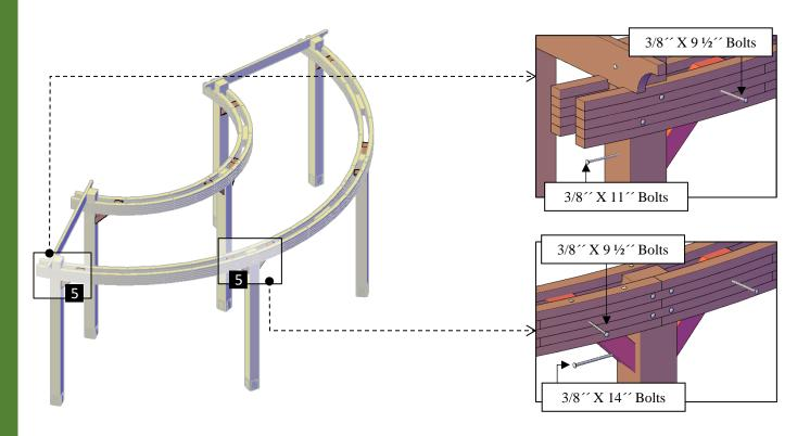
**Step 8:** Use 3/8" x 5" bolts **(H)** to attach the secondary knee braces **(6)** to the perimeter rafters and 3/8" x 10 bolts **(G)** to attach to the posts. Each part has a series of numbers that indicate where to attach the part with the corresponding number.
