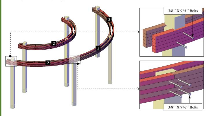
**Step 4:** Use 3/8'' x  $7\frac{1}{2}$ '' bolts **(D)** to attach the supports **(2)** together. Each part has a series of numbers that indicate where to attach the part with the corresponding number.
