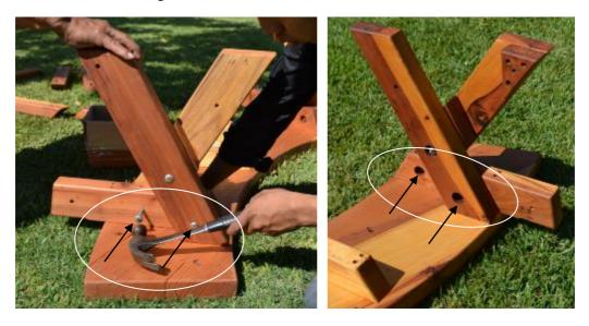
**Step 2:** Turn the seat upside up and attach long leg to seat and short leg with one carriage bolt each. Align the predrilled holes; lightly tap the 2 bolts in. The bolts should tap into their holes. If you have to force a bolt, the leg is probably not oriented properly, is in the wrong hole or it is turned around. Make sure the bolts are tapped all the way into the wood, then add washers and nuts and tighten with a ½-inch ratchet.
