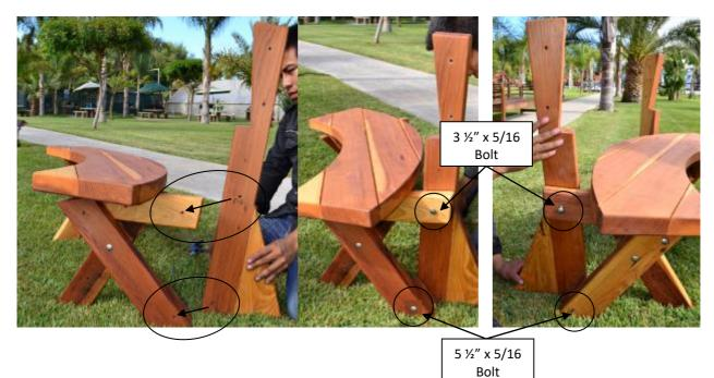
**Step 3**: Attach backrest to long legs with two carriage bolts ( $3 \frac{1}{2}$ " x 5/16), washer and nuts per side. Align the predrilled holes; lightly tap the 2 bolts in. The bolts should tap into their holes. If you have to force a bolt, the leg is probably not oriented properly, is in the wrong hole or it is turned around. Make sure the bolts are tapped all the way into the wood, then add washers and nuts and tighten with a  $\frac{1}{2}$ -inch ratchet.
