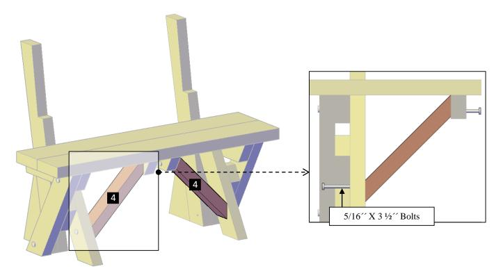
Step 4: Finally, use 5/16" x 3 1/2" bolts (B) to attach the backrest (5) to the long legs. Each part has a series of numbers that indicate where to attach the part with the corresponding number.
