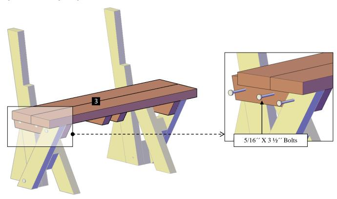
Step 3: Attach the diagonal supports (4) to the short legs and to the seat with 5/16" x 3 1/2" bolts (B). Each part has a series of numbers that indicate where to attach the part with the corresponding number.
