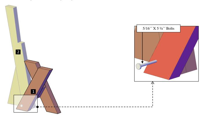
**Step 2:** Attach the seat (3) to the legs with 5/16 x  $3\frac{1}{2}$  bolts (B). Each part has a series of numbers that indicate where to attach the part with the corresponding number.
