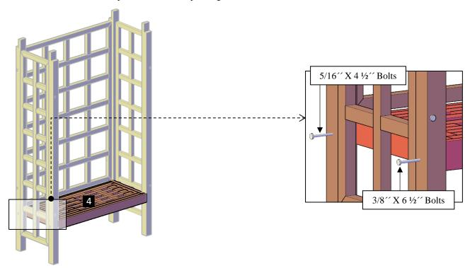
**Step 4:** Use 5/16" X 3" bolts (**C**) to attach the supports (**5**) to the posts. Each part has a series of numbers that indicate where to attach the part with the corresponding number.
