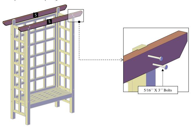
**Step 5:** Attach the back-knee braces **(6)** to the support with 5/16" x 3" bolts **(C)** and to the posts with 3/8" x  $6\frac{1}{2}$ " bolts **(B)**. Each part has a series of numbers that indicate where to attach the part with the corresponding number.
