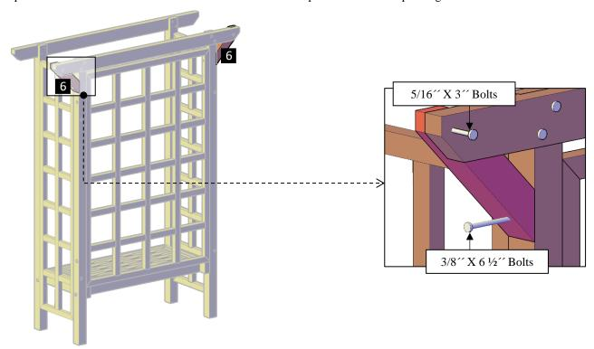
**Step 6:** Attach the front-knee braces (6) to the support with 5/16 '' x 3'' bolts (C) and to the posts with 5/16 '' x 4  $\frac{1}{2}$  '' bolts (A). Each part has a series of numbers that indicate where to attach the part with the corresponding number.
