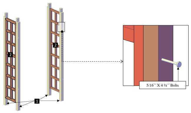
**Step 2:** Use  $5/16^{\prime\prime}$  X  $4\frac{1}{2}^{\prime\prime}$  bolts (**A**) to attach the back-trellis wall (**3**) to the posts. Each part has a series of numbers that indicate where to attach the part with the corresponding number.
