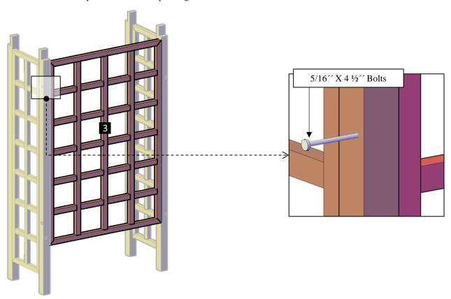
**Step 3:** Attach the seat (4) to the posts with  $5/16^{\prime\prime}$  X  $4\frac{1}{2}^{\prime\prime}$  bolts (A) and  $3/8^{\prime\prime}$  X  $6\frac{1}{2}^{\prime\prime}$  bolts (B). Each part has a series of numbers that indicate where to attach the part with the corresponding number.
