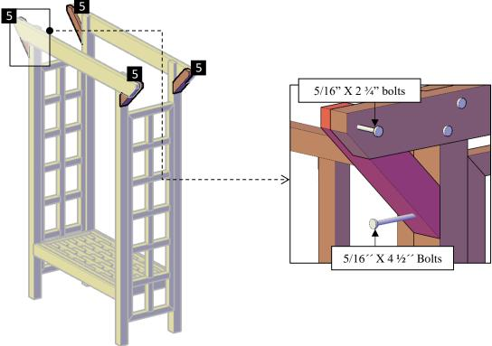
**Step 5:** Finally, use 3" deck screws **(D)** to attach each slat **(6)** to the supports. Each part has a series of numbers that indicate where to attach the part with the corresponding number.
