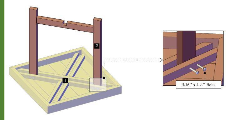
**Step 2:** Attach the second leg (2) to the tabletop with 5/16'' x  $4\frac{1}{2}$ '' bolts (A). The legs will be attached together with  $2\frac{1}{2}$ '' deck screws (B). Each part has a series of numbers that indicate where to attach the part with the corresponding number.
