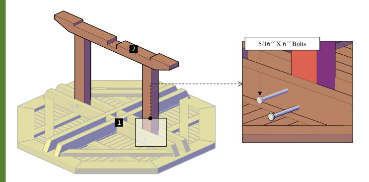
**Step 2:** Attach the other leg (2) to the tabletop with 5/16" x 6" bolts (A). Each part has a series of numbers that indicate where to attach the part with the corresponding number.
