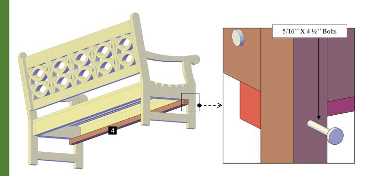
**Step 4:** Use 5/16 '' x  $3\frac{1}{2}$  '' bolts (**C**) to attach the diagonal supports (**5**) to the seat. After that, use 5/16 '' x  $4\frac{1}{2}$  '' bolts (**B**) to attach to the legs. Each part has a series of numbers that indicate where to attach the part with the corresponding number.
