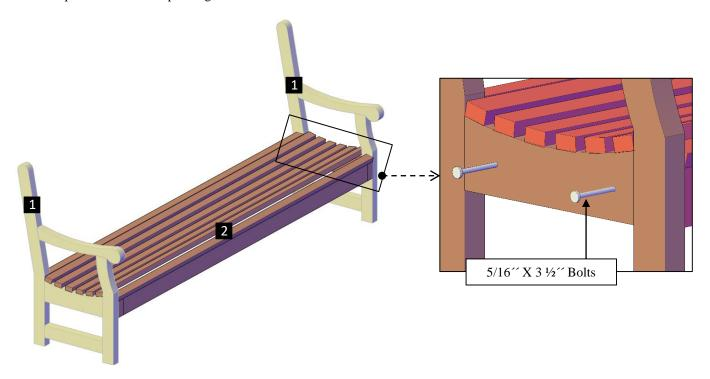
**Step 2:** Attach the backrest (3) to the legs with 5/16 ′′ x  $3\frac{1}{2}$  ′′ bolts (A). Each part has a series of numbers that indicate where to attach the part with the corresponding number.
