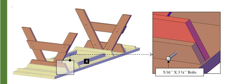
**Step 3:** Use 5/16" x 3 ½" bolts (**B**) to attach the diagonal supports (**5**) to the tabletop and to the legs. Each part has a series of numbers that indicate where to attach the part with the corresponding number.
