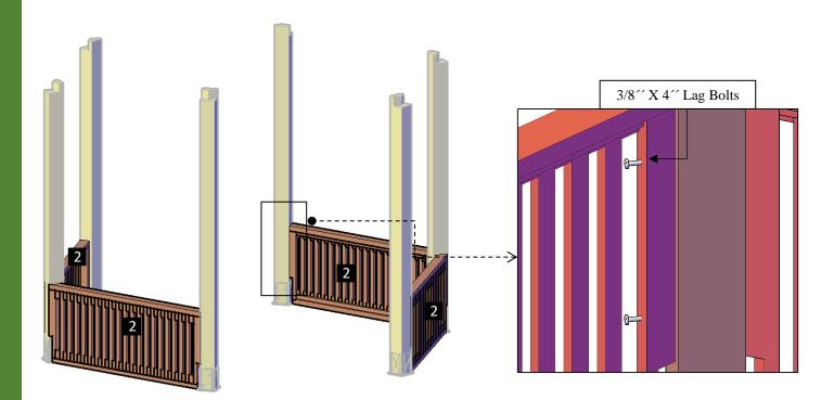
Step 4: Use 3/8 X 4 lag bolts (C) to attach the first frames (3) to the posts. Each part has a series of numbers that indicate where to attach the part with the corresponding number.
