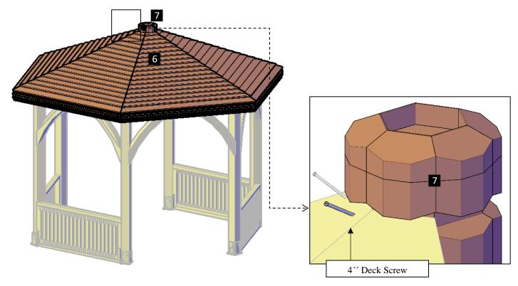
Step 10: Place the tables that were removed from the roof panels. After that, put <u>exterior clear silicone</u> on the roof panels with the second roof frame joints.
