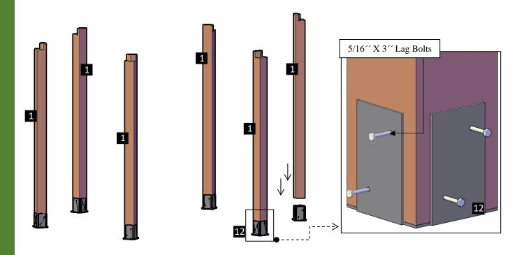
**Step 3:** Use 3/8 ' x 4' lag bolts (C) to attach the fences (2) to the posts. Each part has a series of numbers that indicate where to attach the part with the corresponding number.
