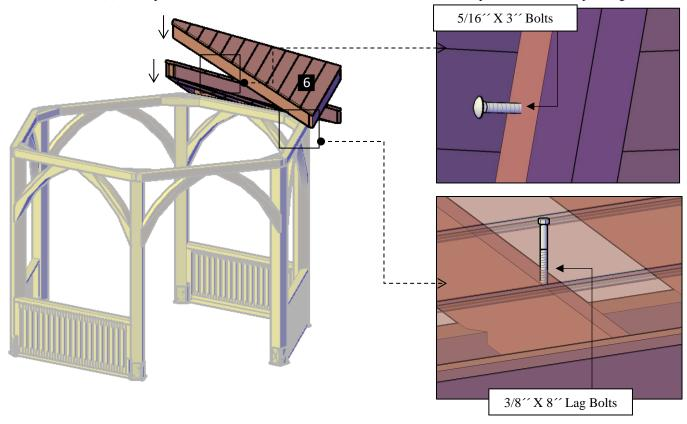
**Step 8:** First, use 5/16 X 3  $\sim$  lag bolts (**B**) to attach the roof panels to second roof base (**7**). Each part has a series of numbers that indicate where to attach the <u>part with</u> the corresponding number.
