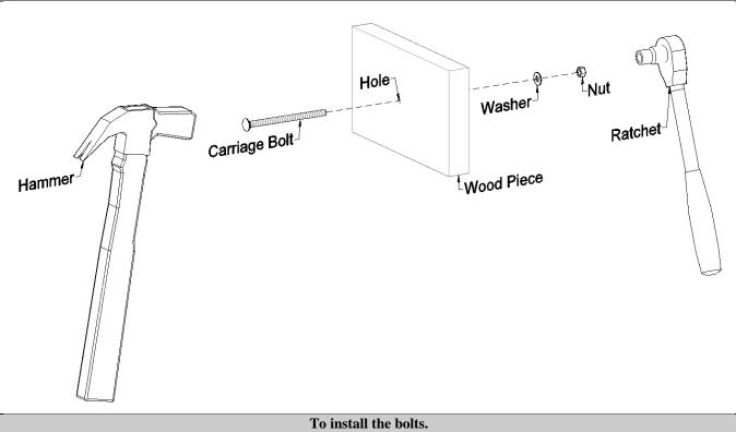
Insert the carriage bolts into the holes and lightly tap with a hammer until the square neck fit in the wood piece and the bolt head must flush with the wood piece. Finally, place the washer and the nut and carefully tighten it using a ratchet with the necessary socket or a wrench.
