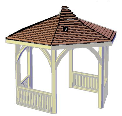
Step 13: Use  $4^{\prime\prime}$  deck screws (H) to attach the roof trims (9) to the roof boards. Each part has a series of numbers that indicate where to attach the part with the corresponding number.
