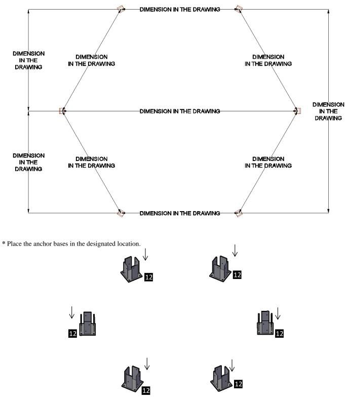
**Step 2:** Set your posts (1) in the saddle of the anchor bases (12). Drill a  $\emptyset \frac{1}{4}$  hole prior to anchoring in each post to facilitate the ratcheting of the hardware. After that, use a 5/16 x 3 lag bolts (**B**) to attach each post to the anchor bases.
