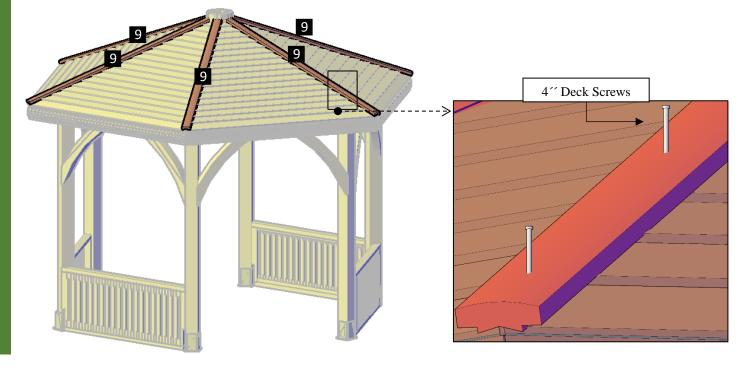
**Step 14:** Insert the second roof (10) in the center of the second roof base. After that, use  $4^{\prime\prime}$  deck screws (**H**) to attach them together. Use  $15/8^{\prime\prime}$  deck screws (**J**) to attach the roof boards for the second roof. Each part has a series of numbers that indicate where to attach the part with the corresponding number.
