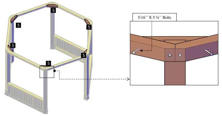
**Step 7:** Use 3/8<sup> $\sim$ </sup> X 8<sup> $\sim$ </sup> lag bolts (G) to attach the roof panels (6) to the first frame. Then attach the roof panels together with 5/16<sup> $\sim$ </sup> X 3<sup> $\sim$ </sup> bolts (F). Each part has a series of numbers that indicate where to attach the part with the corresponding number.
