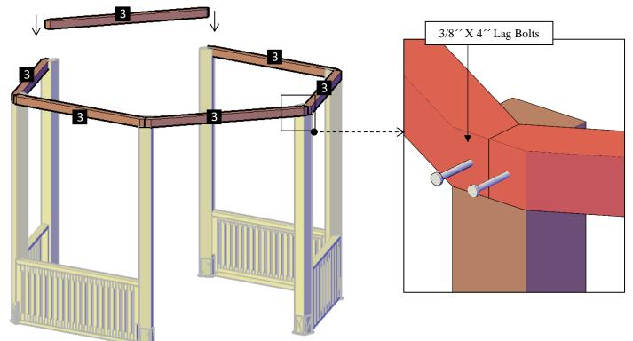
**Step 5:** Attach the braces (4) to posts with 3/8 x 4 lag bolts (C) and to the first frame with 3/8 x 6 bolts (D). Each part has a series of numbers that indicate where to attach the part with the corresponding number.
