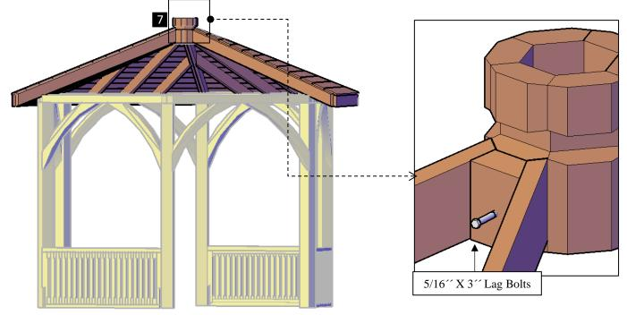
Step 9: Use 4<sup>''</sup> deck screws (H) to attach to the roof panels (6) to the second roof base (7). Each part has a series of numbers that indicate where to attach the part with the corresponding number.
