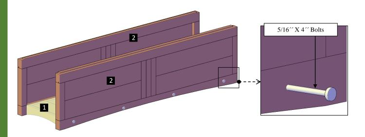
**Step 2:** Attach the short walls (3) to the long walls with  $5/16^{\prime\prime}$  x  $3\frac{1}{2}^{\prime\prime}$  bolts (B), as shown below. Each part has a series of numbers that indicate where to attach the part with the corresponding number.
