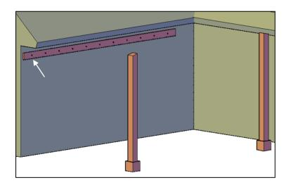
Attach the Ledger board to the house with lag bolts (5/16" x 3") one every 16" on center
