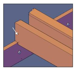
Attach the supports to the ledger board with deck screws (3" x 8") at 45 degree angles to attach to the supports. Two deck screws per support
