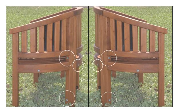
**Step 3:** Attach the front brace to sides. The predrilled holes have numbers written on them on the interior side. Match these numbers to the numbers written next to the holes on the front brace piece. Tap the 4½-inch carriage bolt from the outside in. Tap the bolt in all the way, then add washers, nuts and tighten with ½-inch ratchet. Do not overtighten.
