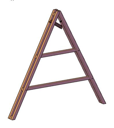
**Step 6:** Use 3/8" X 10" Bolts (**A**) with washer and nut to attach the top main supports (**3**) to the frame legs. Each part has a series of numbers that indicate where to attach the part with the corresponding number.
