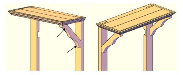
**Step 3:** Attach Hanger Board to leg assembly left, with deck Screws (6"x 1 5/8") *Repeat to the other side.*
