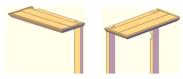
**Step 2:** Attach Cantilever Support to part leg assembly right, with four Deck Screws (8"x 3") *Repeat with the other cantilever support.*
