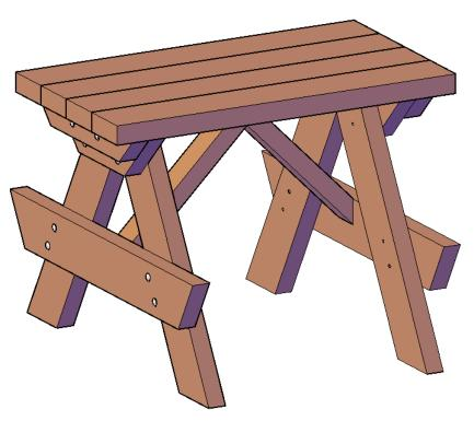
**Step 4:** Finally, use 5/16" x 3 ½" bolts (**A**), washers (**B**) & nuts (**C**) to attach the benches (**4**) to the legs. Each part has a series of numbers that indicate where to attach the part with the corresponding number.
