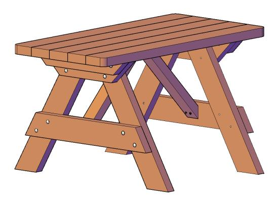
**Step 4:** Place the seat upside down. After that, use  $5/16^{\prime\prime}$  x  $3\frac{1}{2}^{\prime\prime}$  bolts (A), washers (B) & nuts (C) to attach the legs (5) to the seat (4). Each part has a series of numbers that indicate where to attach the part with the corresponding number.
