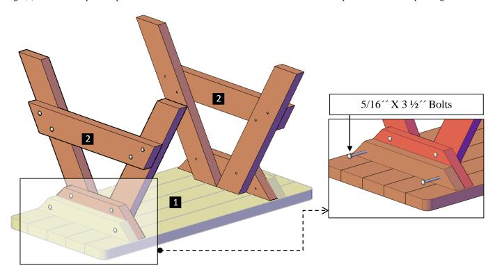
**Step 2:** Attach the knee braces (3) to the tabletop and to the legs with 3" deck screws (**D**). Each part has a series of numbers that indicate where to attach the part with the corresponding number.
