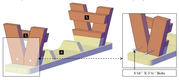
**Step 5:** Attach the diagonal supports **(6)** to the legs and to the seat with 5/16" x 3 ½" bolts **(A)** or 3" deck screws **(D)**. Each part has a series of numbers that indicate where to attach the part with the corresponding number.
