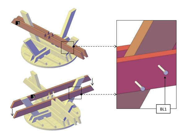
**Step 3:** Turn tabletop over its feet. After that, attach the benches (**5**) to the cross supports with 3/8" x 5" bolts (**BL1**). Each part has a series of numbers that indicate where to attach the part with the corresponding number.
