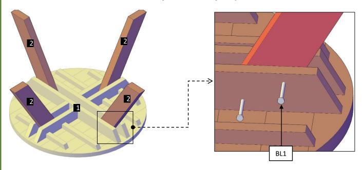
**Step 2:** Use 3/8" x 5" bolts (**BL1**) to attach the cross supports (3) to the legs. Each part has a series of numbers that indicate whereto attach the part with the corresponding number.
