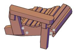
**Step 2:** Attach backrest to armrests with 2 bolts washer and nuts per side. Match the numbers next to the predrilled holes on the backrest to the numbers on the chair side. Tap the carriage bolts all the way into the wood, then attach the washers, nuts and tighten with ½-inch ratchet. Do not over-tighten.
