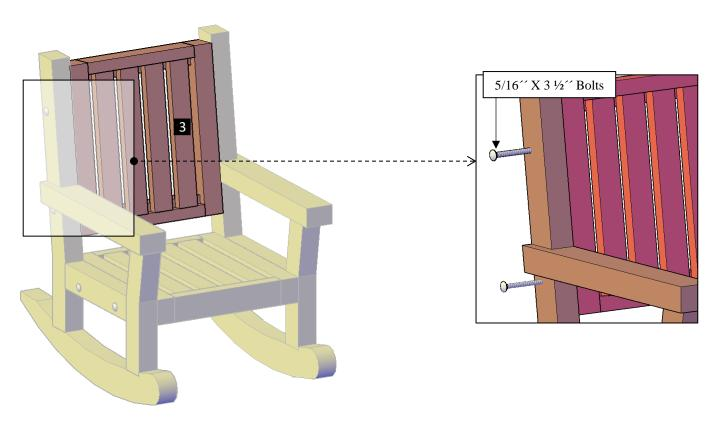
Step 3: Finally, use 5/16" x 3 1/2" bolts (B) with washers (B) & nuts (C) to attach the support (4) to the legs. Each part has a series of numbers that indicate where to attach the part with the corresponding number.
