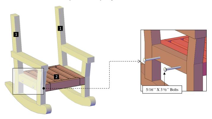
**Step 2:** Attach the backrest (3) to the legs with 5/16 'x  $3\frac{1}{2}$  'bolts (A), washers (B) & nuts (C). Each part has a series of numbers that indicate where to attach the part with the corresponding number.
