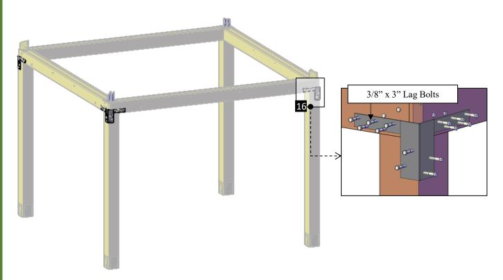
**Step 7:** Use 5/16 ′′ x  $3 \frac{1}{2}$  ′′ bolts (**G**) to attach the diagonal rafters (**4**) to the metal plaques. After that, attach the diagonal rafters to the cupola frame (**5**) with 3/8 ′′ x 10 ′′ lag bolts (**C**). Each part has a series of numbers that indicate where to attach the part with the corresponding number
