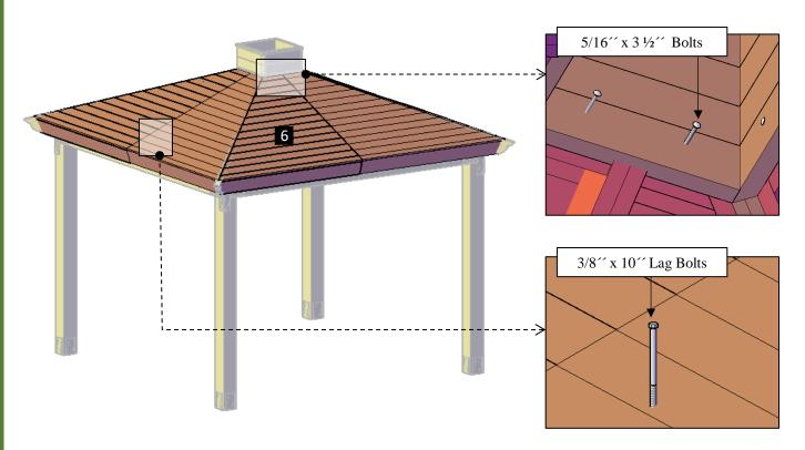
**Step 9:** Attach the roof panels (6) to the diagonal rafters with 3/8" x  $3\frac{1}{2}$ " lag bolts (H). The roof panels will be attached together with 5/16" x 3" bolts (I). Each part has a series of numbers that indicate where to attach the part with the corresponding number.
