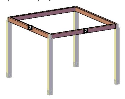
**Step 3:** Attach the single supports (3) to the posts and to the supports with in-between blocking with 3/8" X 10" lag bolts (C). Each part has a series of numbers that indicate where to attach the part with the corresponding number.
