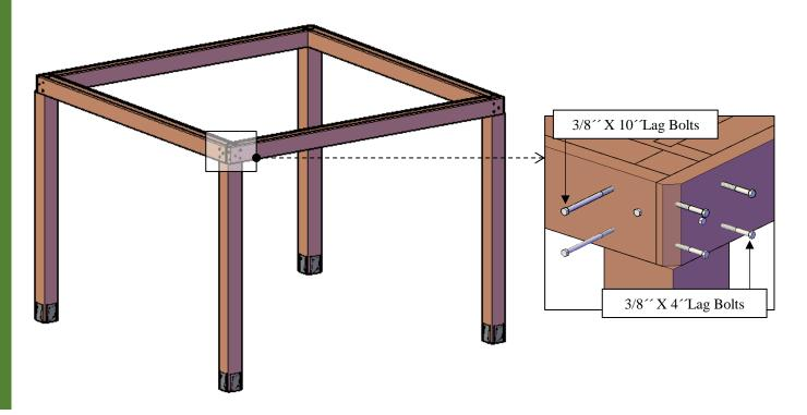
Step 5 Attach the single supports to the supports with in-between blocking, use 3/8" x 7" bolts (E)4E3.
