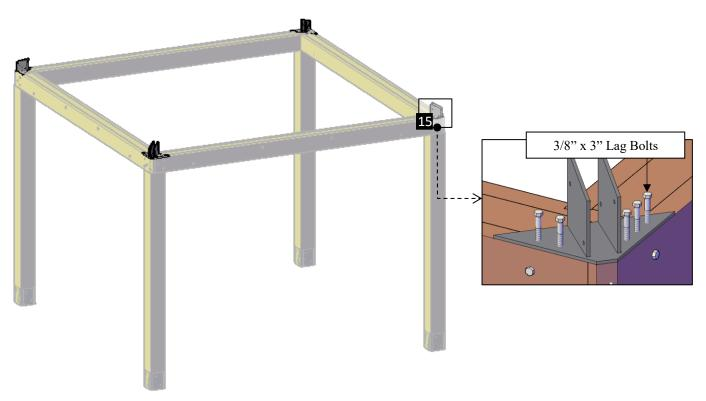
**Step 6:** Use 3/8" x 3" lag bolts (**F**) to attach the T-Supports (**16**) to the posts and to the supports. Each part has a series of numbers that indicate where to attach the part with the corresponding number.
