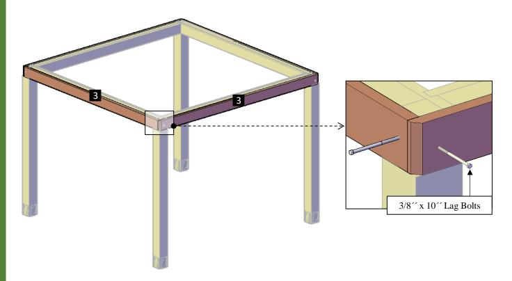
**Step 4:** Attach the single supports to the supports with in-between blocking, use 3/8 '  $\times 10$  ' lag bolts (**C**) and 3/8 '  $\times 4$  ' lag bolts (**D**).
