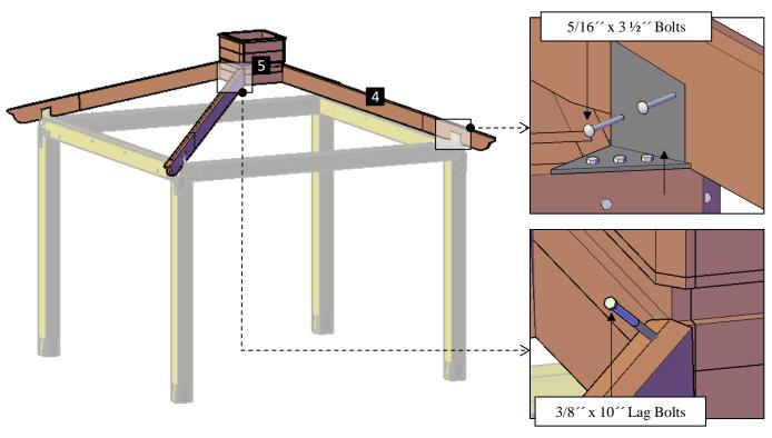
**Step 8:** Use 3/8" x 10" Lag bolts (**C**) to attach the roof panels (**6**) to the supports and 5/16" x 3 ½" bolts (**G**) to attach to the cupola frame. Each part has a series of numbers that indicate where to attach the part with the corresponding number
