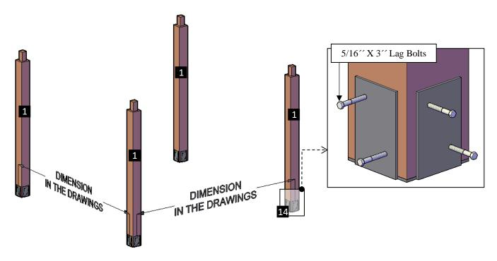
**Step 2:** Put up the supports with in-between blocking (2), into the post notches as shown. Each part has a series of numbers that indicate where to attach the part with the corresponding number.
