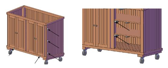
**Step 5:** Attach top to side walls with 2 carriage bolts  $(4" \times 5/16")$ , washers and nuts per side. Match the numbers written next to the predrilled holes.
