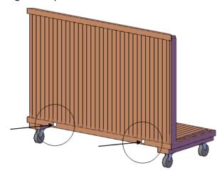
**Step 2:** Attach side wall to back wall with 3 carriage bolts (2 ½" x 5/16"), washers and nuts. Line up the predrilled holes on both sides and make sure the numbers written match. *Repeat this step for other side wall.*
