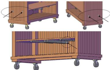
**Step 4:** Attach front wall to side walls, shelves and floor. Use two carriage bolts (4" x 5/16), washers and nuts to attach to floor, 3 carriage bolts (2  $\frac{1}{2}$ " x 5/16"), washers and nuts to attach to each side wall and one carriage bolt (3" x 5/16") to attach to each shelf
