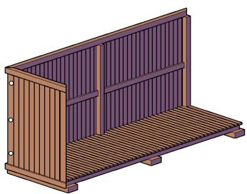
**Step 3:** Attach shelf to walls. Use two carriage bolts (3" x 5/16"), washers and nuts to attach to each side wall and one carriage bolt, washer and nut to attach to back wall as shown below. Repeat this step for the other shelf.
