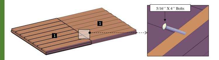
**Step 2:** Attach the long walls (2) to the floor, with bolts 5/16 ' x 4' bolts (A), as shown below. Each part has a series of numbers that indicate where to attach the part with the corresponding number.
