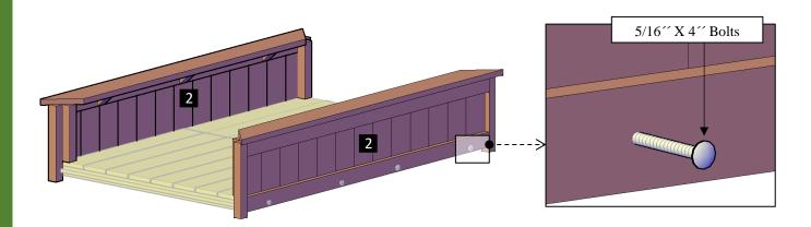
**Step 3:** Attach the short walls (3) to the floor with 5/16" x 4" bolts (**A**) and, attach the short walls to the long walls with 5/16" X 2 ½" bolts (**B**), as shown below. Each part has a series of numbers that indicate where to attach the part with the corresponding number
