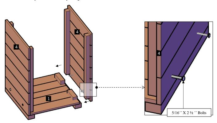
**Step 2:** Attach the short walls (3) to the other walls with  $5/16^{\prime\prime}$  X 2  $\frac{1}{2}^{\prime\prime}$  Bolts (A). Each part has a series of numbers that indicate where to attach the part with the corresponding number.
