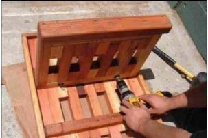
\*Small bench legs are attached at the edge of the seat as shown below:
