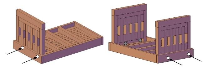
**Step 2:** Attach the diagonal support to the leg and underside of bench seat with the stainless steel screws supplied. The holes have already been drilled. Use a #2 square bit to screw the stainless steel 2 ½ inch screws into the four pre-drilled holes (if you don't have a no. 2 square bit, you can pick one up at any hardware store for \$1). Repeat this step with the other side.
