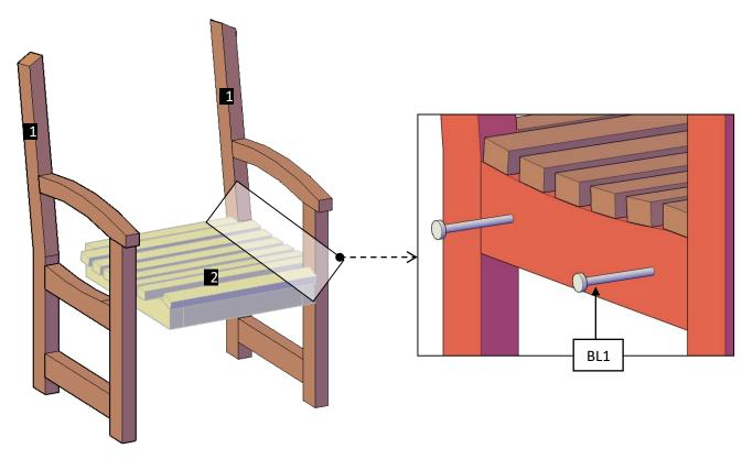
Step 2: Attach the backrest (3) to the legs with  $5/16^{\prime\prime} \times 3\frac{1}{2^{\prime\prime}}$  bolts (BL1). Each part has a series of numbers that indicate where toattach the part with the corresponding number.
