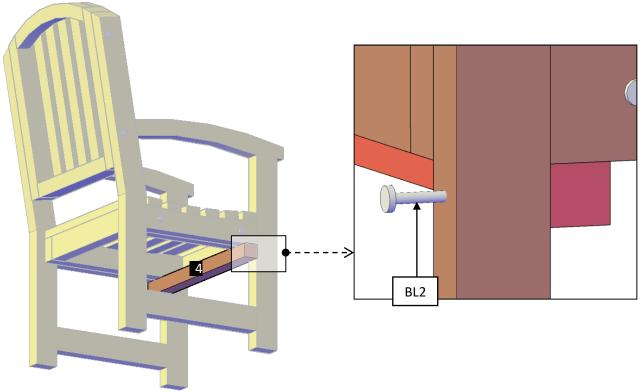
**Step 4:** Use  $5/16^{\prime\prime} \ge 3\frac{1}{2}^{\prime\prime}$  bolts (**BL1**) to attach the diagonal supports (**5**) to the seat. After that, use  $5/16^{\prime\prime} \ge 4\frac{1}{2}^{\prime\prime}$  (**BL2**) bolts to attach the legs. Each part has a series of numbers that indicate where to attach the part with the corresponding number.
