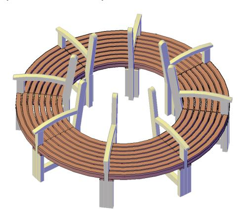
**Step 3:** Finally, attach the Backrests (3) to the legs with 5/16 x  $5 \frac{1}{2}$  bolts (A). Each part has a series of numbers that indicate where to attach the part with the corresponding number.
