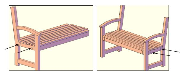
**Step 2:** Attach part D (arm assembly right) to part B (Backrest), with two bolts (3 ½" x 5/16"), washers & nuts (into two holes marked "3"). Tap the bolt all the way into the wood to set it. Then add a washer and nut and lightly tighten.
