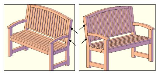
**Step 3:** Attach diagonal supports to seat & sides with two bolts, washers & nuts each one. Tap the bolt all the way into the wood to set it. Then add a washer and nut and lightly tighten.
