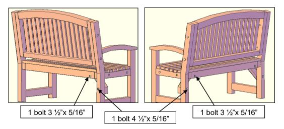
**Step 4:** Attach front brace to sides, with one bolt ( $4 \frac{1}{2}$ " x 5/16"), washer & nut per side. Tap the bolt all the way into the wood to set it. Then add a washer and nut and lightly tighten.
