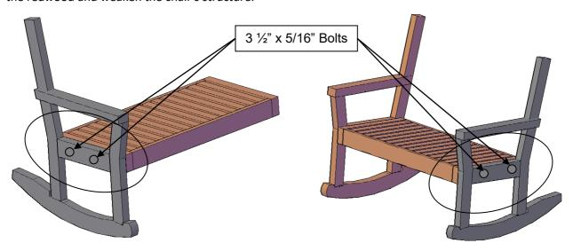
**Step 2:** Attach backrest to arms with 2 bolts, washers and nuts per side. Match up the numbers written next to the holes. Tap the 4 carriage bolts all the way into the wood and through both the arms and the chair seat. Then insert the washers and nuts from the interior side of the chair seat and tighten with a ½-inch ratchet. Do not over tighten or you'll crush the redwood and weaken the bench's structure.
