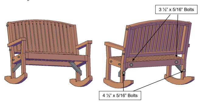
**Step 4:** Attach front support to arms with 2 bolts, washers and nuts. Match the numbers next to the predrilled holes on the interior of the arms to the numbers on the front support. Tap the carriage bolts all the way into the wood, then attach the washers, nuts and tighten with ½-inch ratchet. Do not overtighten.
