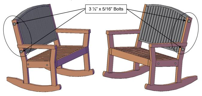
**Step 3:** Attach diagonal supports to seat & arms (2 bolts per support). Match the numbers next to the predrilled holes on the back rest to the numbers on the back rest supports on each chair side. Tap the carriage bolts all the way into the wood, then attach the washers, nuts and tighten with ½-inch ratchet. Do not over-tighten.
