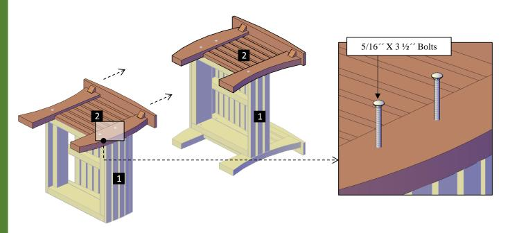
**Step 2:** Turn the chair over its feet. Finally, attach the backrest (3) to the legs, use  $5/16^{\prime\prime}$  x  $3\frac{1}{2}^{\prime\prime}$  bolts (A) &  $5/16^{\prime\prime}$  x  $6\frac{1}{2}^{\prime\prime}$  bolts (B) with washers and nuts. Each part has a series of numbers that indicate where to attach the part with the corresponding number.
