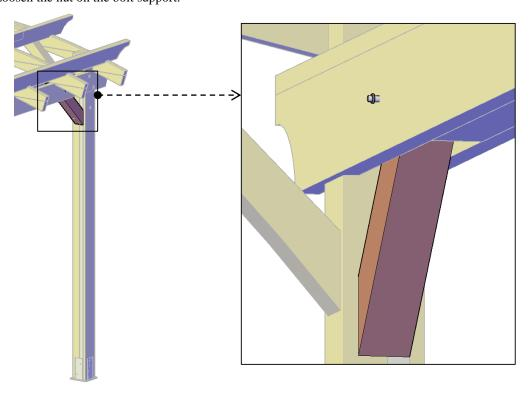
**Step 3:** The bolt of the post and the brace must be flush with the post.
