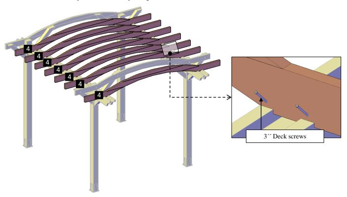
**Step 9:** Attach the slats **(8)** to the arched rafters with 3" deck screws **(E)**. Each part has a series of numbers that indicate where to attach the part with the corresponding number.
