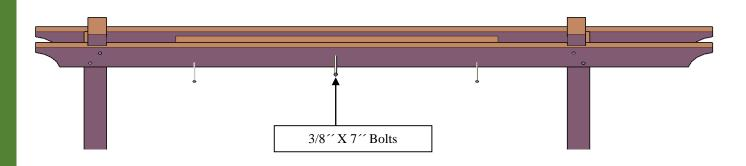
**Step 5:** Attach the perimeter arched rafters first (4) to the posts with 3/8" x 6" bolts (**D**) and to the supports with 8" x 3" deck screws (**E**). Each part has a series of numbers that indicate where to attach the part with the corresponding number.
