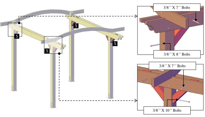
**Step 7:** Attach the secondary knee braces (6,7) to the posts with 3/8" x 10" bolts (G) and to the arched rafters with 3/8" x 5" bolts (H). Each part has a series of numbers that indicate where to attach the part with the corresponding number.
