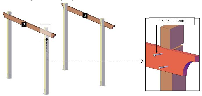
Step 3: Place the supports with in-between blocking (3), into the post notches as shown and attach to the post with the single support bolts. Each part has a series of numbers that indicate where to attach the part with the corresponding number.
