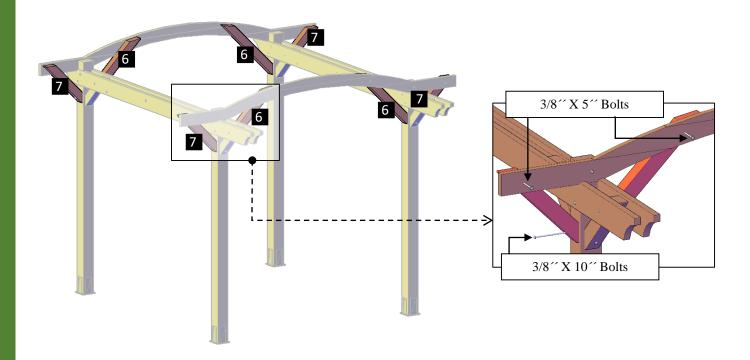
**Step 8:** Use 8" x 3" deck screws (**E**) to attach the other arched rafters (**4**) to the supports. Each part has a series of numbers that indicate where to attach the part with the corresponding number.
